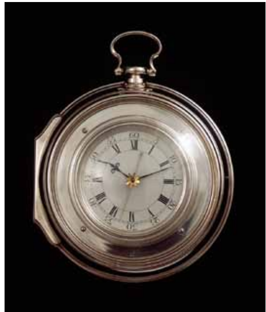
The fifth marine timekeeper (H5) made by John Harrison and completed in 1770. Photo Clockmakers' Company, © National Maritime Museum.
