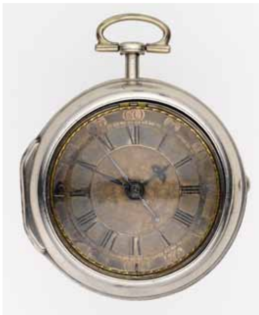
A centre-seconds stop-watch with cylinder escapement by George Graham, believed to have been made for the third Astronomer Royal, James Bradley ©NMM
