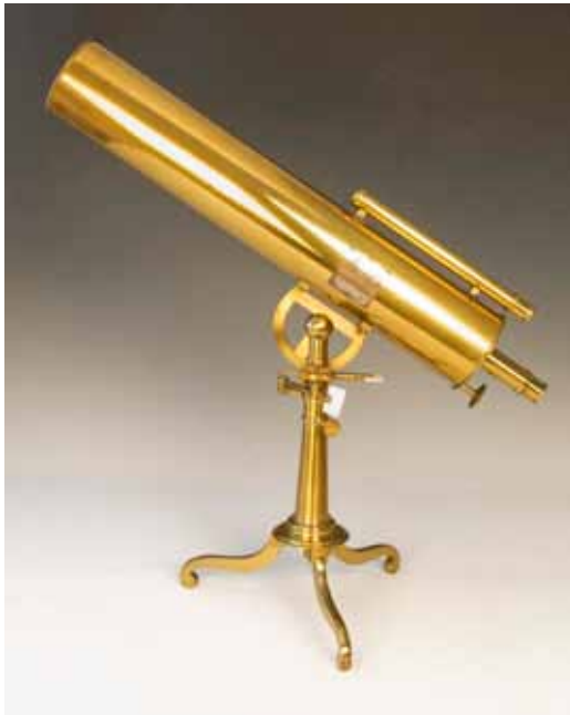
This fine telescope, with its altazimuth stand was donated to Magdalen College, Oxford, in 1755. It was made by James Short (1710-68), ‘optician, solely for reflecting telescopes’. Primary and secondary mirrors in speculum metal. Focus by screw moving secondary, long rod and knurled knob at eye-end. Museum of the History of Science, Oxford, lent by Magdalen College.
