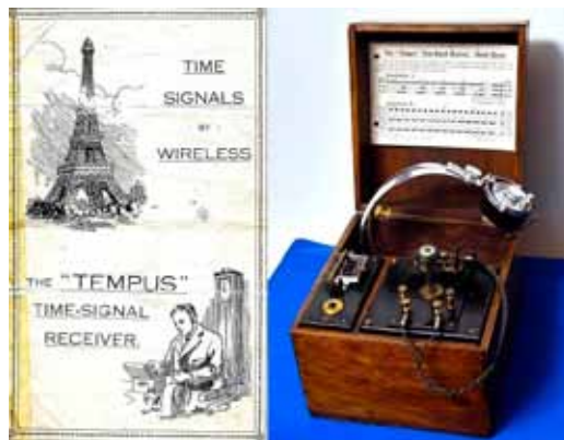
The Tempus time signal receiver, here shown with its instruction manual, was manufactured specifically for time signal reception from the Eiffel Tower.
