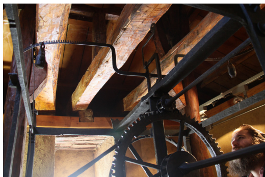
One of the two known turret clocks in Spain still retaining their pre-pendulum escapements. Santa Marina del Rey town hall (Leon), 1590.
