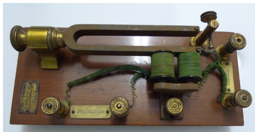
Electrically-maintained tuning fork for timing physiological experiments by G. Boullitte, Paris, c. 1890. From the laboratory of Jacques Arsène d'Arsonval, Paris.
