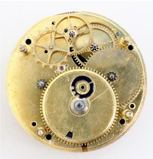
Fig. 15. The train of the Russell-Cotes movement showing the going barrel and cylinder escape wheel. (Dale Sardeson)
