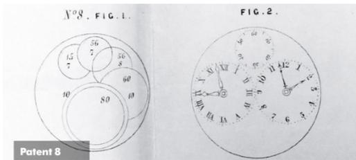
Fig. 5. Patent No.8. Leslie's design for the dual dial of the Nautical Watch (Rich Newman).
