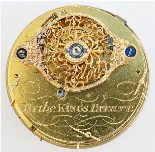
Fig. 8. The upper plate of the Russell-Cotes movement. The balance bridge is signed by Joseph Dodds in the piercing (Dale Sardeson)
