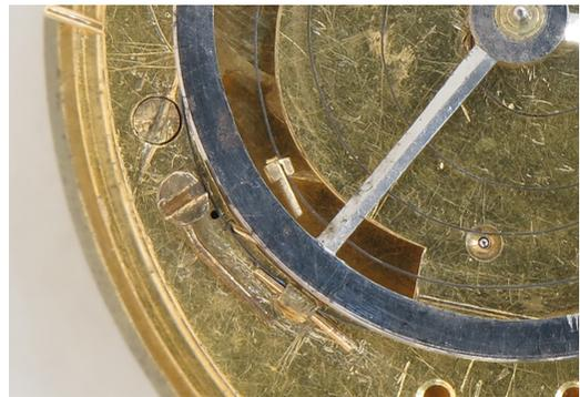
Fig. 17. View onto the upper plate showing the brass arm pinned to the last turn of the balance spring and the brass regulating screw with brass pin, on the left - should be turned through 180 degrees to act alongside the outer turn of the balance spring. (Dale Sardeson)
