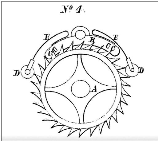
Fig. 4. Leslie's constant-force clock escapement (Patent No. 4), employing impulsing springs mounted on the pallet frame, with rollers acting on the escape wheel teeth (Rich Newman).
