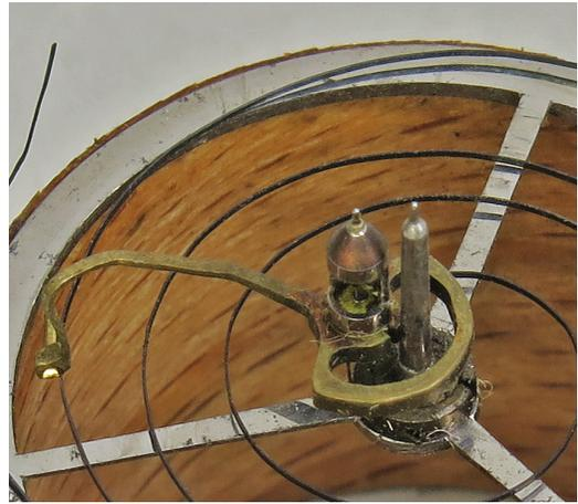
Fig. 16. The cylinder mounted alongside the balance staff, but only connected to the balance via the brass arm, impulsing through the balance spring. The photo was taken before conservation cleaning. (Dale Sardeson)
