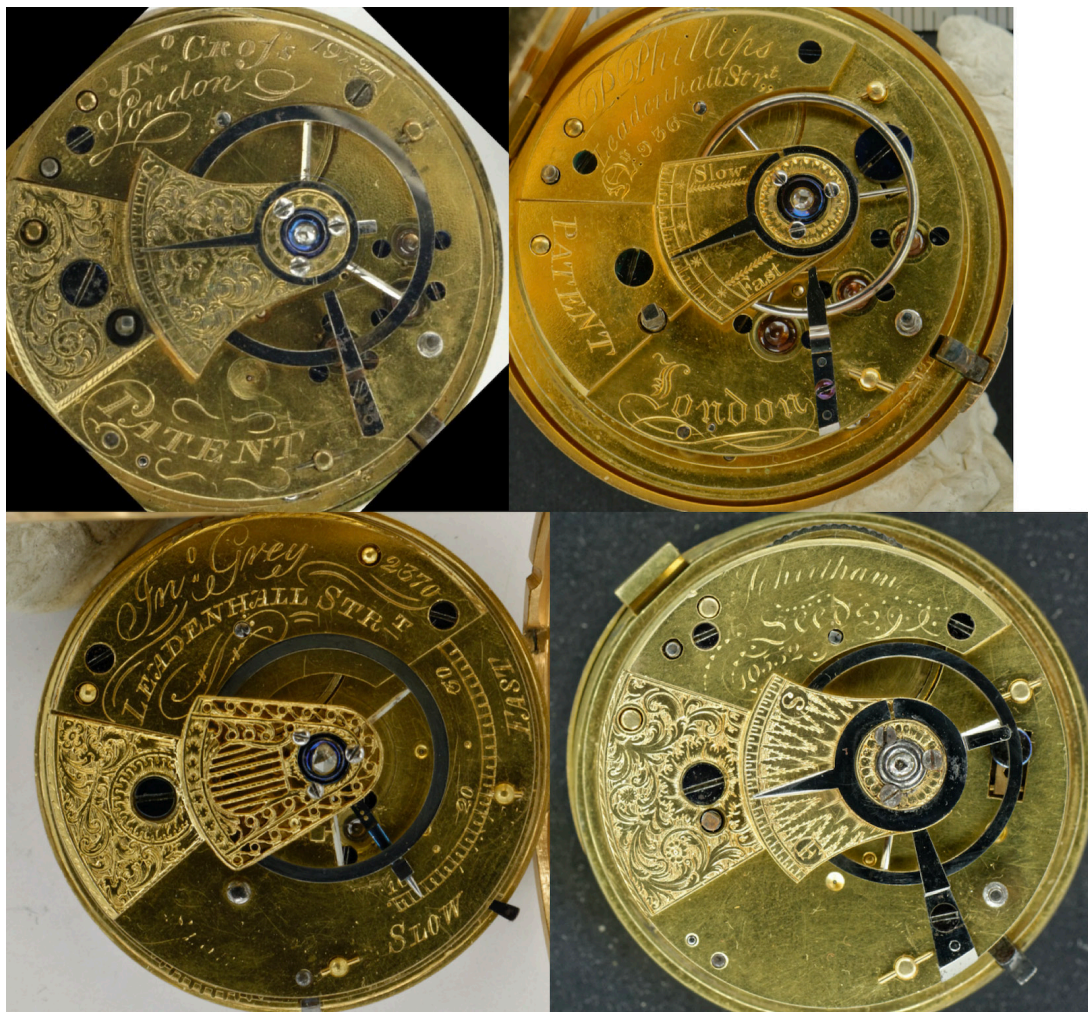
Fig. 13, London-finished rack levers. Top left , John Cross, London, written 'Patent' on the top plate. No slides. Oversprung; lever 'scape and 4 th jeweled. Top right Phillip Phillips, in a gold pair case dated 1817. Slides to the lever. Oversprung. Lower left Jonathan Grey in a gold consular case marked for 1825. Not marked 'Patent', no slides. Steel pallets and a gold escape wheel. Lower right , Cheetham, Leeds, in silver pair cases marked for 1809. Not marked 'Patent'. Oversprung.
