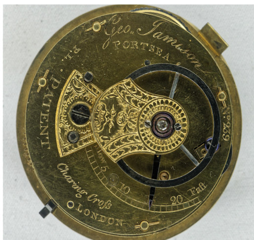
Fig. 9. A London rack lever signed for George Jamison and marked P.L. Patent on the top plate. In silver hunting case marked for London, 1801.
