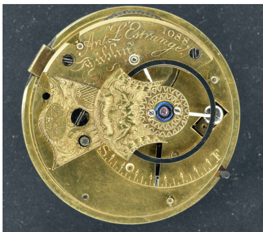
Fig. 8b. Anthony L'Estrange, Dublin 1088 in a gold case marked for Chester 1804. On the cockfoot is written 'Patent P.L.' and Litherland's serial number, 3075, is scratched on the reverse.
