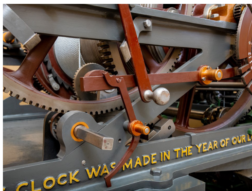
Fig. 11. Original stop levers for the hand-winding process. Image Lumen Photography.
