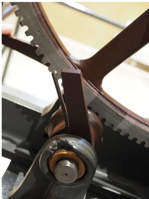
Fig. 10. The damper spring is pressed up against one of the arms, when locked. Image: Andrew Strangeway.
