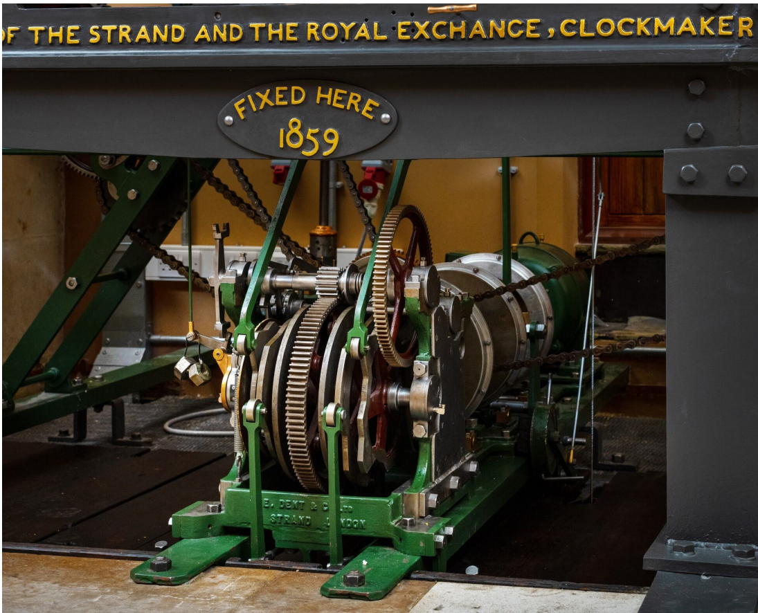
Fig. 17. The mechanism back in position below the clock, ready for testing. Image Lumen Photography.
