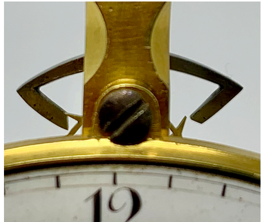
Fig. 15. The constrained design of the dead-beat escapement allows only for a small supplementary arc before bottoming. The exit pallet (left) has just received the escape wheel tooth but has very little further to go before reaching the root of the wheel teeth. (Jonathan Betts)
