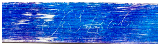
Fig. 10. The high-quality, tapered mainspring is signed: 'RS 1806' and is probably contemporary with the clock's creation. (Jonathan Betts)
