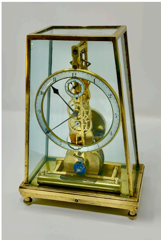
Fig. 7. Signed by William Nicholson, the little skeletonised clock was intended to be mounted in gimbals and to be portable. The tiny square on the front of the base unlocks the glass cover (Jonathan Betts).
