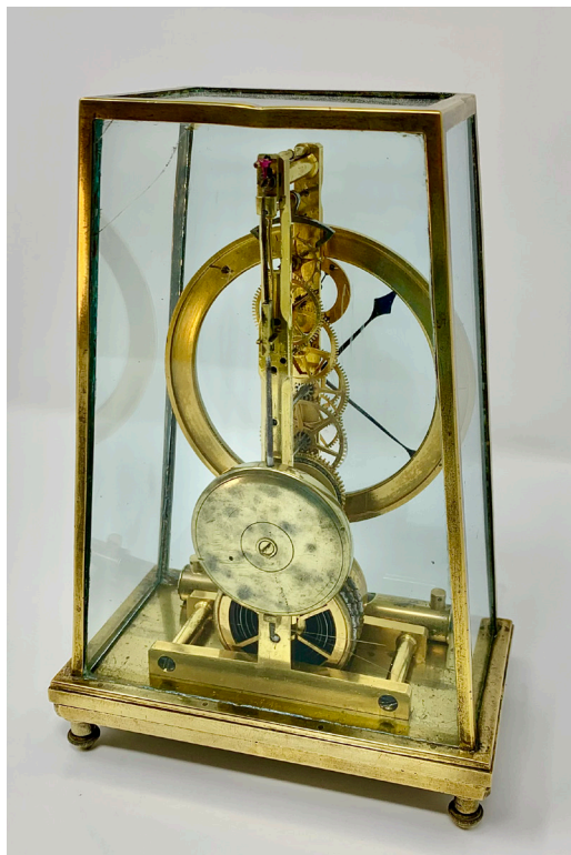
Fig. 8. The rear view of the clock, showing the later pendulum and open mainspring barrel (Jonathan Betts).
