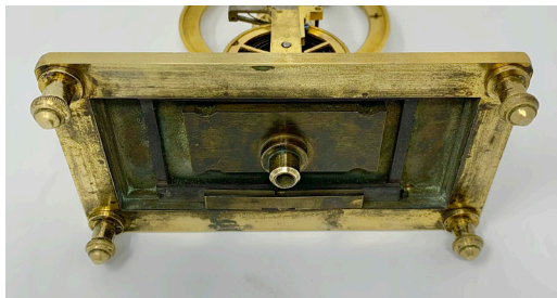
Fig. 12. The base has a threaded socket for fitting a weighted rod to keep the clock horizontal when in its gimbal mounting. (Jonathan Betts)
