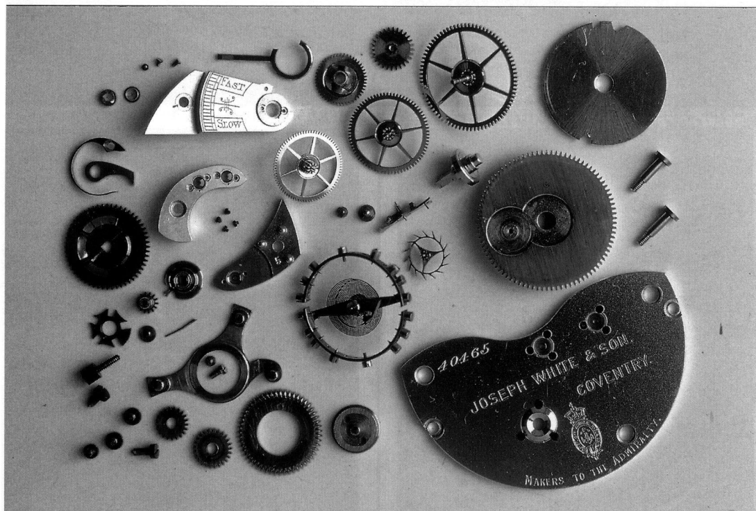
Fig. 16. Movement components No. 40465. Courtesy Anthony G. Randall.
