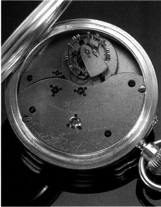
Fig. 8. Joseph White & Son's 'Six-Minute Flying Tourbillon' No. 38715, the back plate. © Sotheby's.
