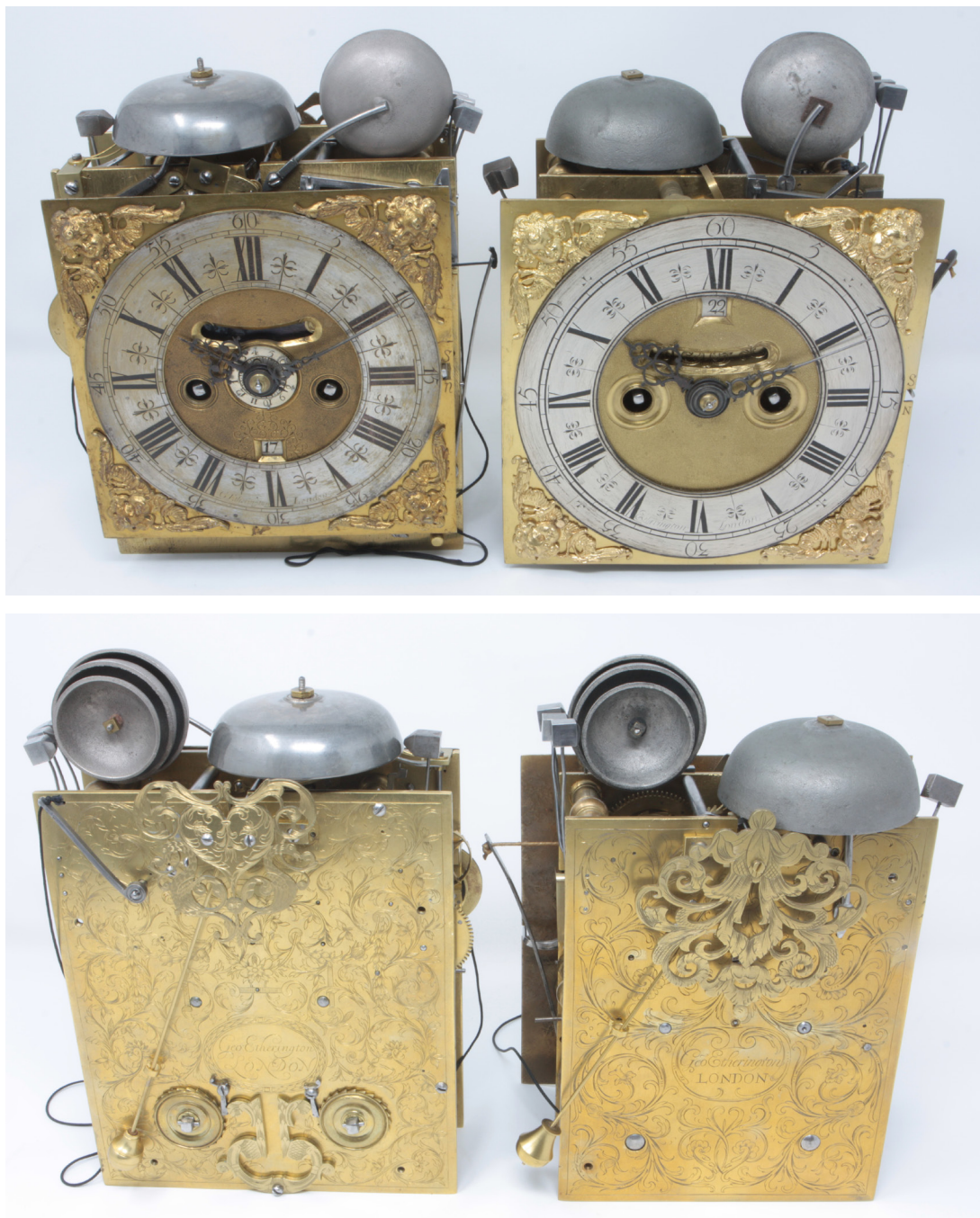
Figs 23a and b. George Etherington 1690s (L) Quare movement (R) Windmills movement.
