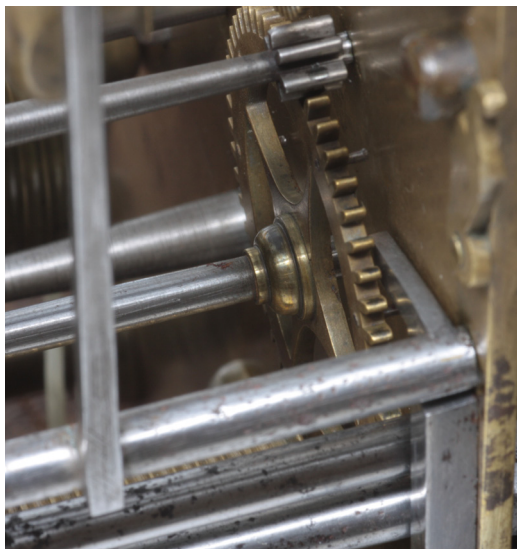
Fig. 12. Collets (R) Clement spring clock (L) East longcase movement from Clement's workshop.
