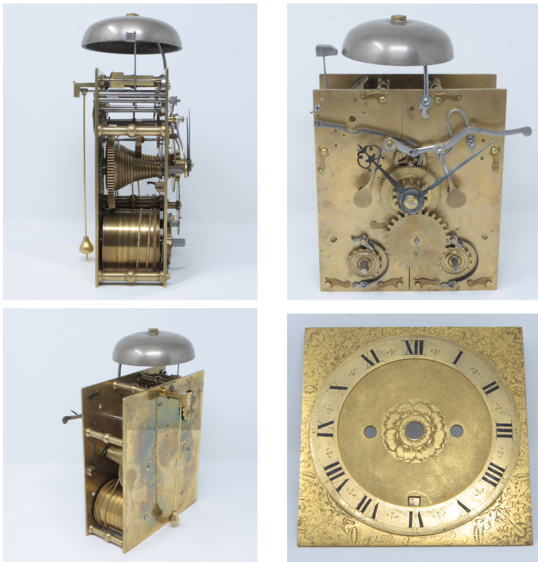
Fig. 8. Split-plate movement 1666–70 with gilt dial signed East.
