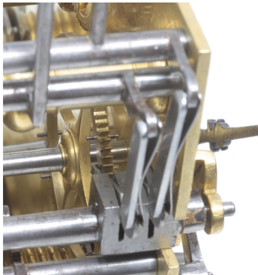
Fig. 12. Collets (R) Clement spring clock (L) East longcase movement from Clement's workshop.
