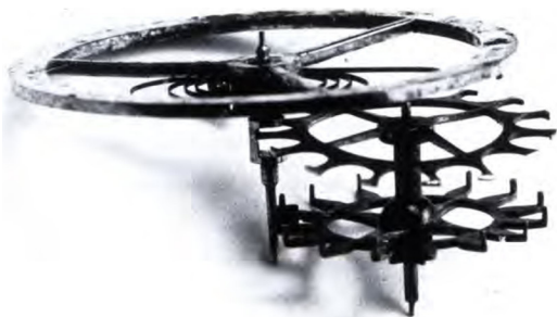
Fig. 11. Pierre Le Roy's escapement with two escape wheels.
