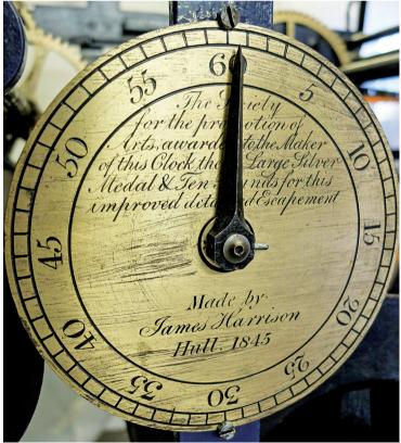
The detached escapement is really a gravity escapement, not a grasshopper as it might seem on first glance. In operation each pivoted two-part pallet is raised into its closed position by the locking escape wheel. On unlocking the pallet gives impulse to the pendulum by hinging into its open position.
