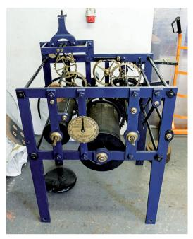
Cast iron was used extensively by James 4 in his clocks for the frames, train bars and great wheels. He later used cast iron skeleton dials. The pendulum bob is under the clock to the left, the clock beats 2 seconds and the semi arc is large, about 5 degrees.
