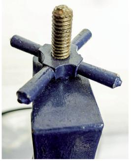
Regulation is achieved from the top of the pendulum. A hand nut raises or lowers the pendulum, the suspension spring slides through a fixed slot. Note the peculiar hollow cone centres that are a hallmark of Harrison's turned work.
