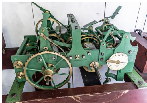
The movement of the floral clock in Hesketh Park, Southport, Sefton, signed on the setting dial by James Ritchie, Edinburgh. The floral clock dates from 1936, and in 2010 it was replanted to the 1930s design.
