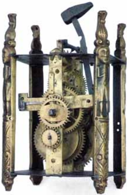
Fig. 3. Movement from the front with replaced hour wheel and pinion of report to increase the duration. Note the single screw hole near the centre of each front pillar for fixing the dial. The purpose of the two screw holes in the right-hand rear pillar is not known.
