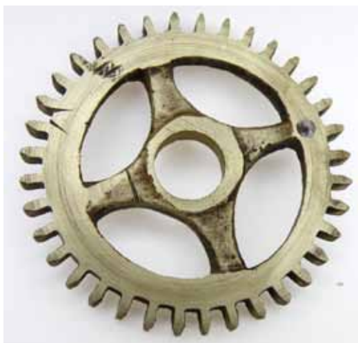
Fig. 11. The hour wheel with alignment marks (left) and an iron pin filed flush that indicate its former use as a reverse minute wheel, possibly from a very small turret clock. The crossings are of an unusual section for a clock.
