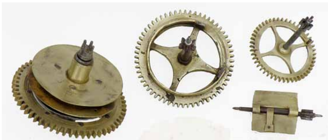
Fig. 7. The striking train, showing the four-pronged pinion of report. The fly is later.
