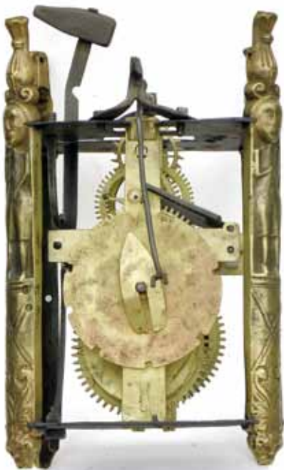
Fig. 4. Rear view with the later iron backcock and crutch after conversion to anchor escapement.
